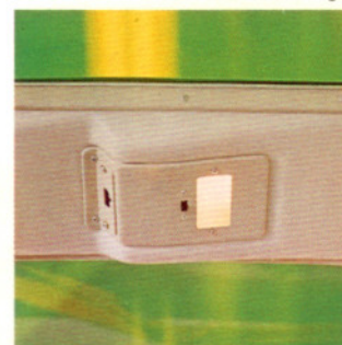
Overhead Dome Light
